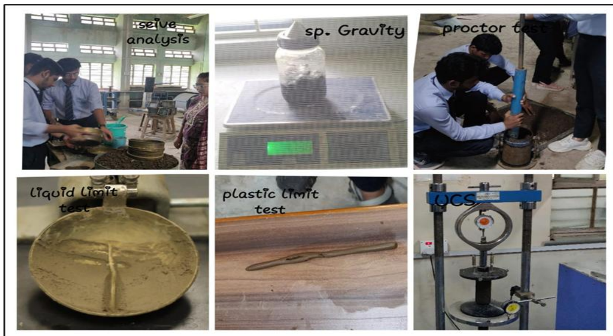
Figure 2: Different testing on prepared soil sample
