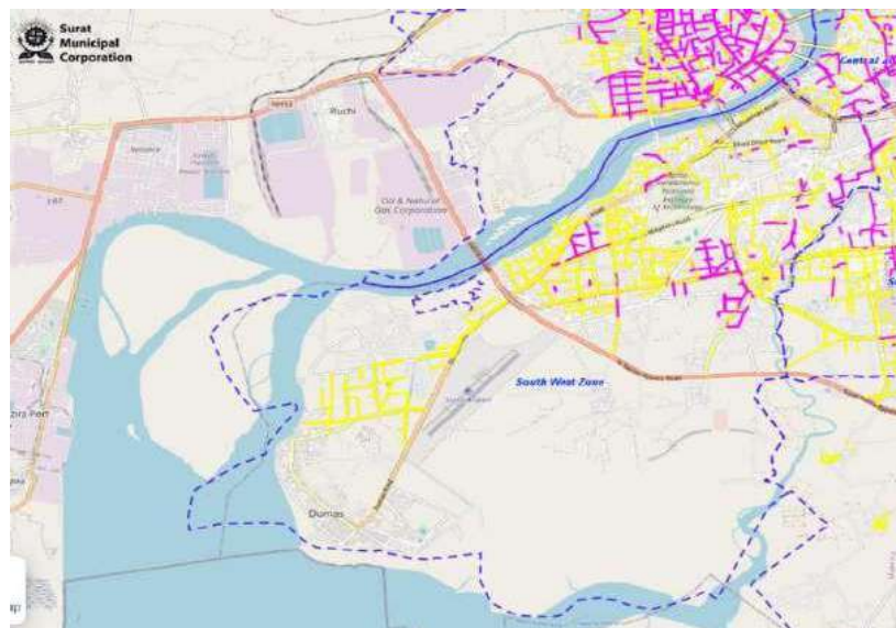
Fig 5.1 Stormwater Drainage Network
