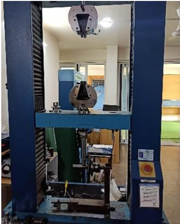
Fig.37 Specimen under compression test using UTM. Testing Graph
