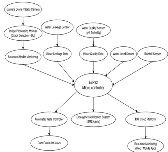
Figure 2. Flowchart of the Proposed Techno Dam
