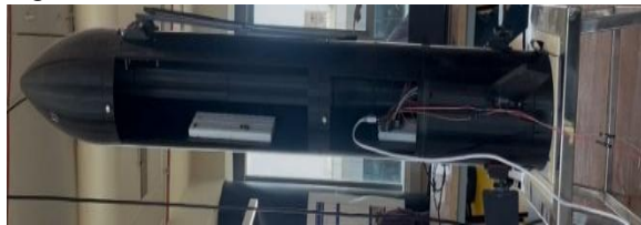
Figure 3: Fabricated inert model of the SDB
