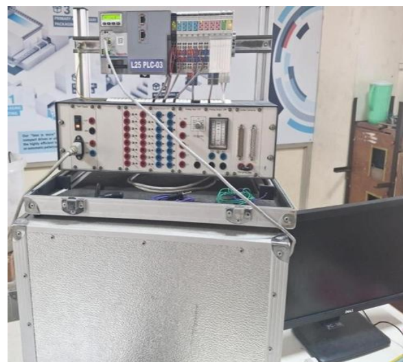
Fig 5: Prototype of the System (PLC Unit)
