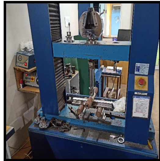
Fig. Specimen under flexural test using a UTM.
