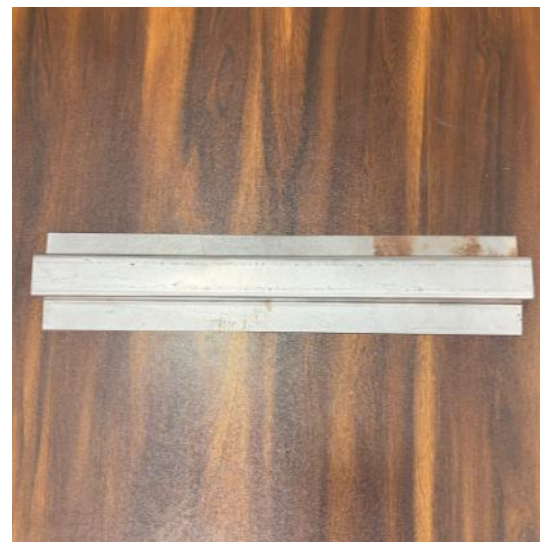
Fig. Final manufactured Hat type side door anti-intrusion beam.
