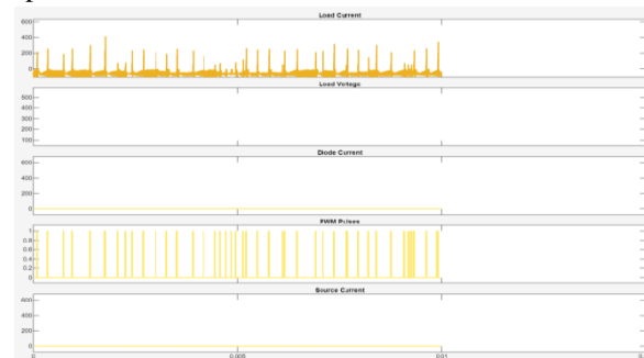
Figure 6. Simulated waveforms showing load current, load voltage, diode current, PWM pulses, and bus current in the BLDC motor control system
