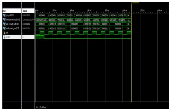
Fig 1. Simulation Output Waveform Analysis of 8-bit MIPS Single-Cycle Processor
