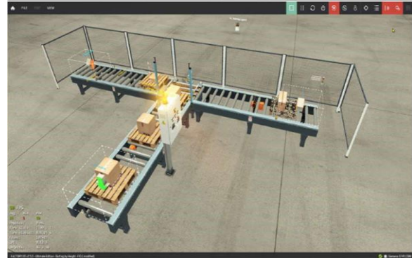
Fig 2. 3D Simulation of The Baggage Sorting System
