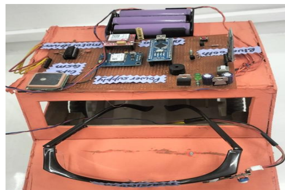
Fig.2 shows a real built Bluetooth car hardware prototype. Arduino Nano is installed into the center of
