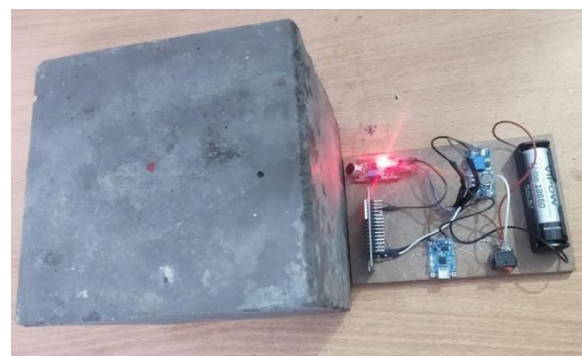
Figure 6.3 Prototype for Concrete Performance Monitoring
