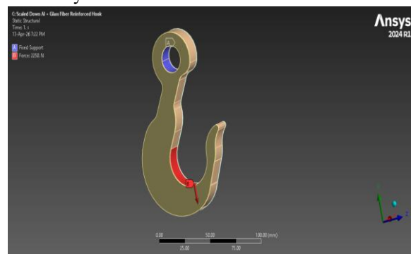
Fig. Boundary conditions for Static Structural Analysis of the GFR Al Hook prototype.
