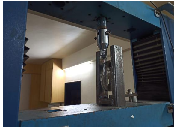
Fig. Specimen under compression test using UTM.
