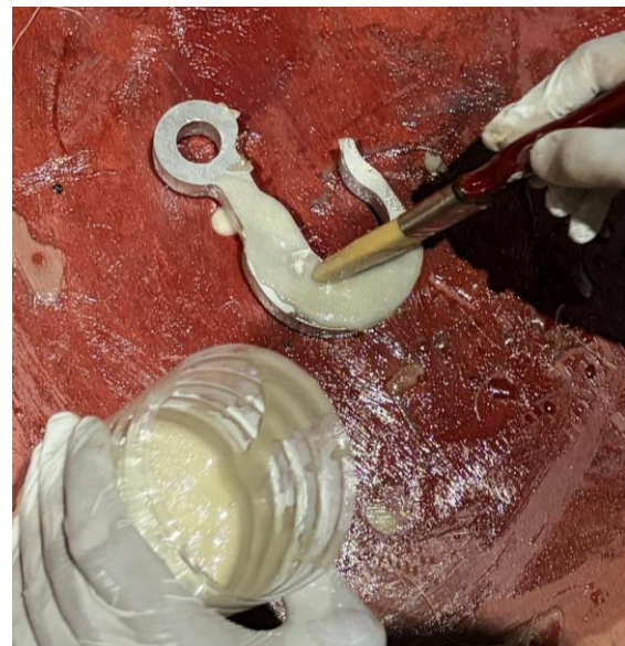
Fig. Reinforcement of glass fiber composite using Resin solution.
