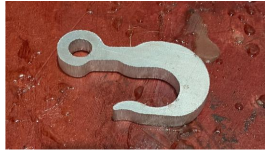
Fig. Aluminium crane hook prototype after waterjet cutting.
