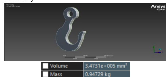
Fig. Geometry of Aluminium Glass Fiber reinforced Crane Hook.
