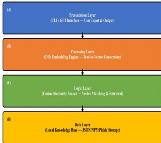
Fig. 1. System architecture diagram illustrating the four-layer modular structure: (a)Presentation Layer with CLI/GUI interface, (b)Processing Layer with Dlib embedding engine, (c)Logic Layer with cosine similarity search, and (d)Data Layer with local knowledge base storage.
