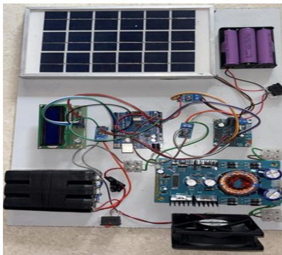
Fig 6. Hardware of a high-gain converter
