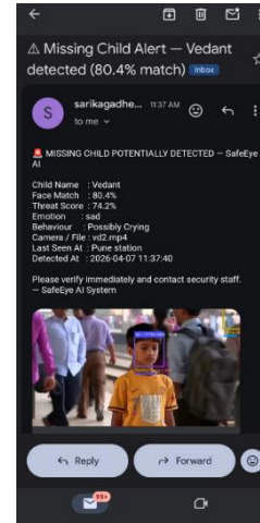
Fig. 2: Automated email alert sent to guardian upon successful face match with snapshot attachment.
