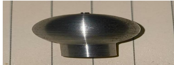
Fig 2: pipe union blanking
