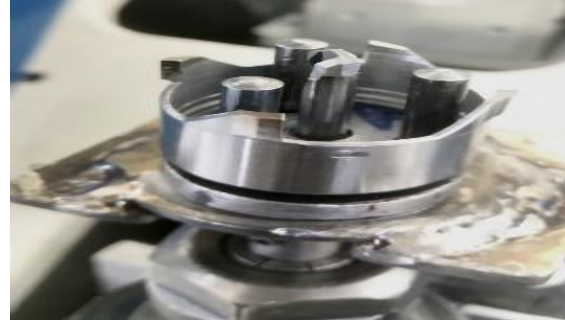
Figure 4. customized HSS 4point drill bit
