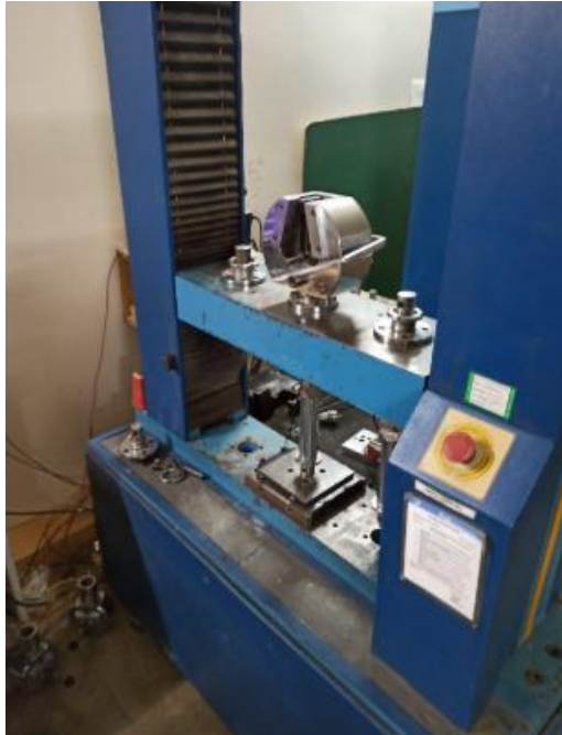
Fig. Specimen under compression testing using UTM.
