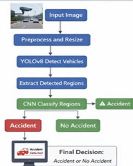
Fig. 4. Flowchart of the Proposed YOLO + CNN Accident Detection Methodology
