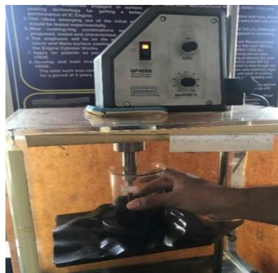
FIGURE 3. Illustrates dispersion of CNTs using ultrasonication technique
