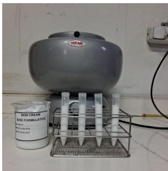
Figure 13: Centrifuge test – emulsion stability test
