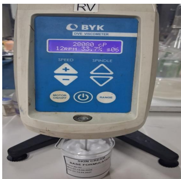
Figure 14: Brookfield viscometer viscosity test
