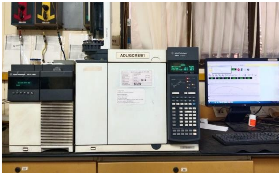
Figure 11: Agilent Technologies 5977A-MSD GC-MS system used for phytochemical profiling.
