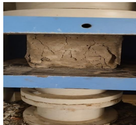
Fig.2: Compressive strength test of cube using CTM
