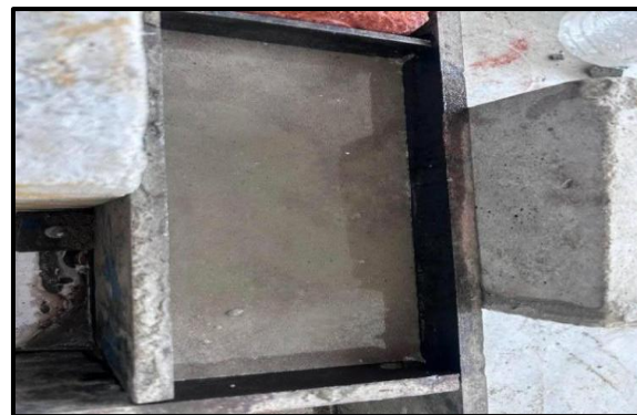
Fig 5 Shows Moulding of Brick
