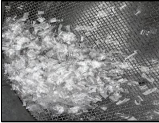
Fig (2) shows shredded Plastic
