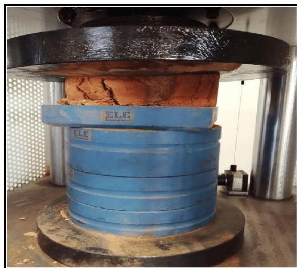
Fig 6 Compression Test Conducted for Clay Plastic Bricks
