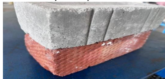
Fig no.1 Plastic bricks Sample (plastic and clay)
