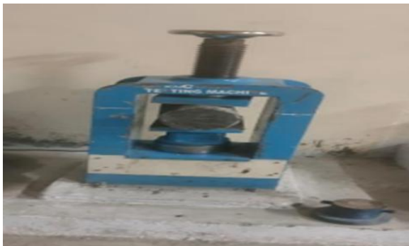
Fig -4: Cylinder Testing
