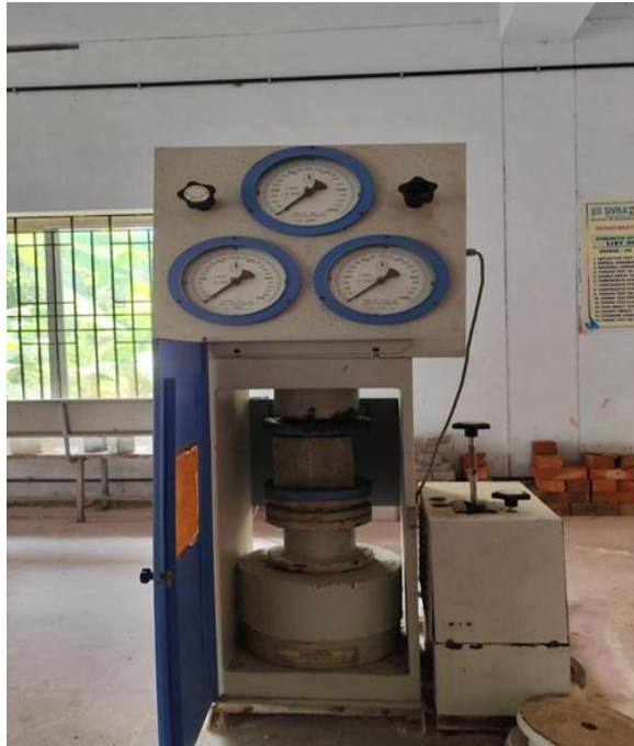
Fig.1 Compression strength test
