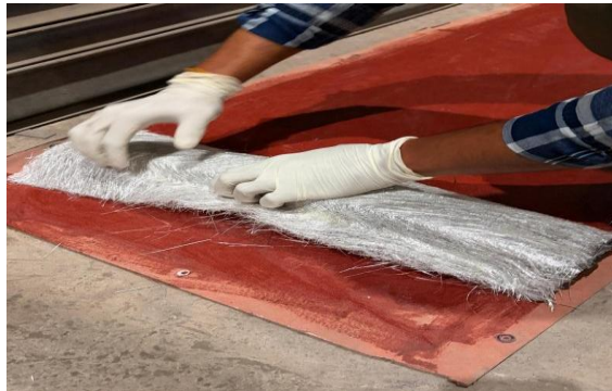
Fig. No.7.1: B-Pillar with Glass Epoxy Reinforcement for Testing
