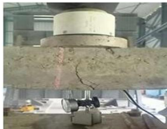
Fig.9. Cracks on the RC beam
