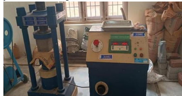
Fig.5. Compressive strength test
