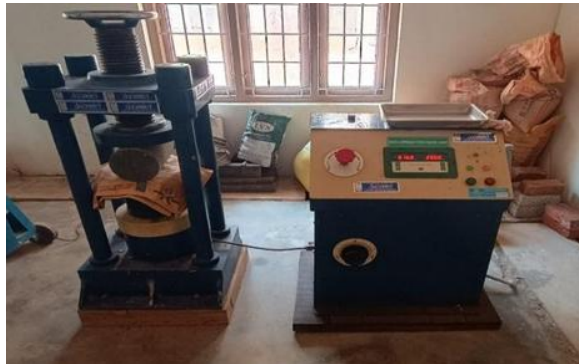
Fig.7. Split tensile strength test
