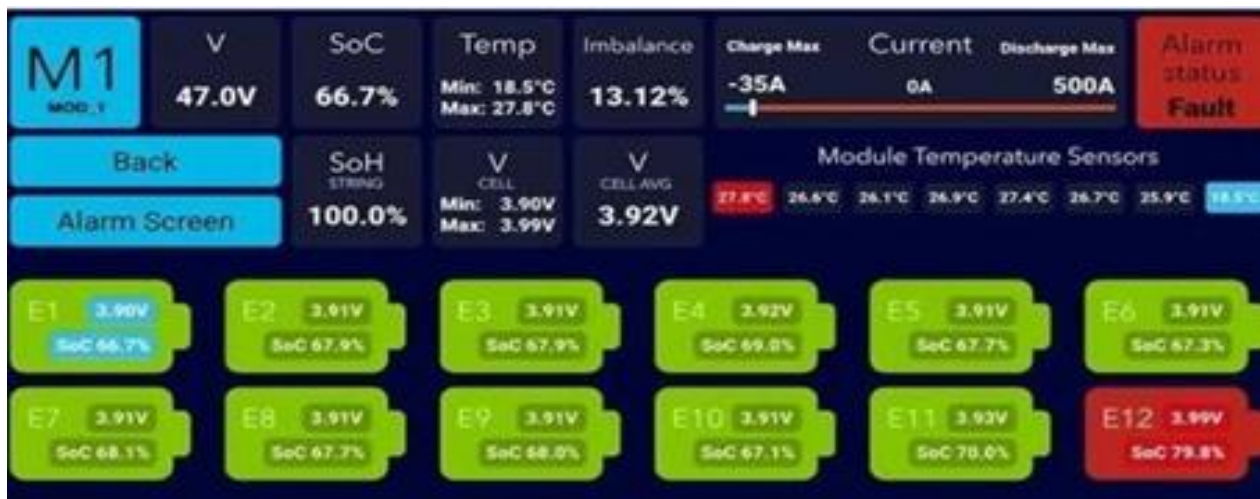
Fig:1 Dashboard of the industrial BMS
