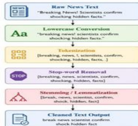
Fig. 2. NLP preprocessing stages used for fake news detection.
