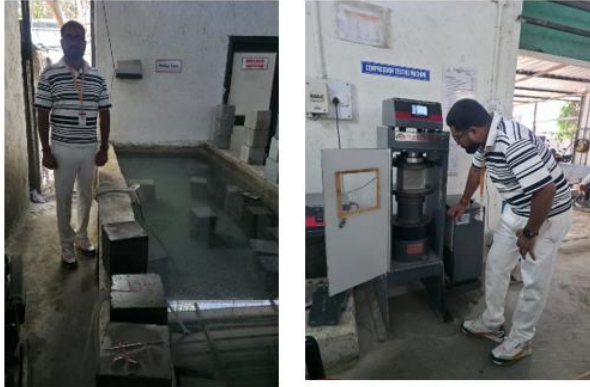
Fig 3 Curing and testing of cube
