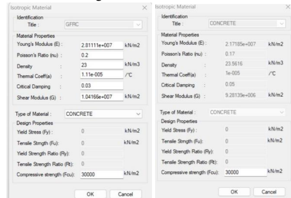
Figure 5.4: Material Property Definition in STAAD.Pro
