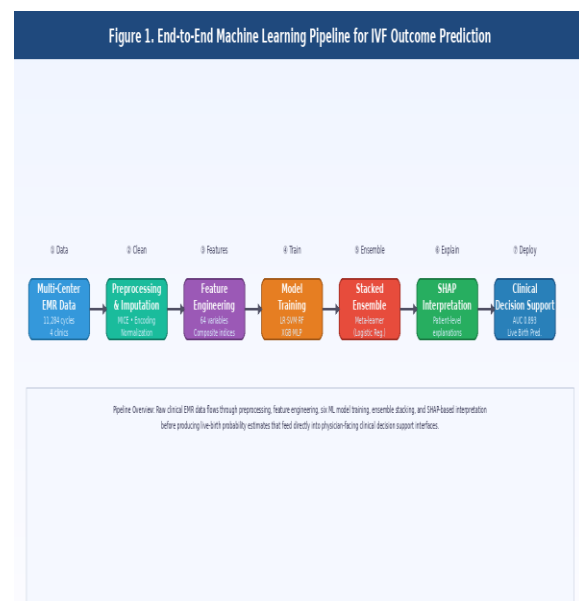
Figure 1. End-to-end machine learning pipeline from multi-center EMR data ingestion through preprocessing, feature engineering, model training, ensemble stacking, SHAP interpretation, and clinical decision support integration.
