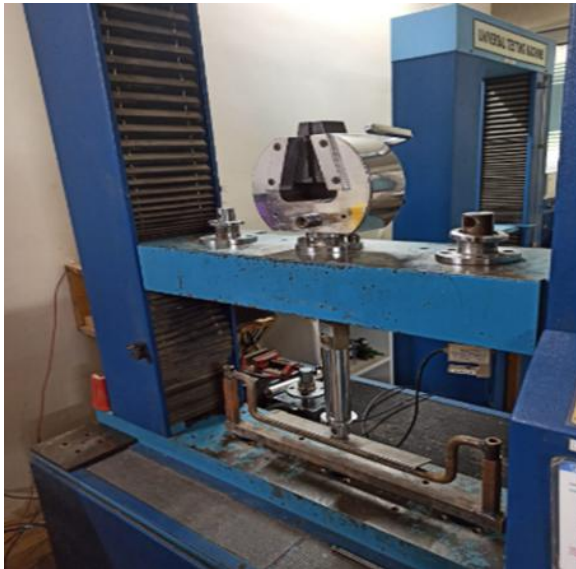
Fig 22. Specimen under compression test using a UTM
