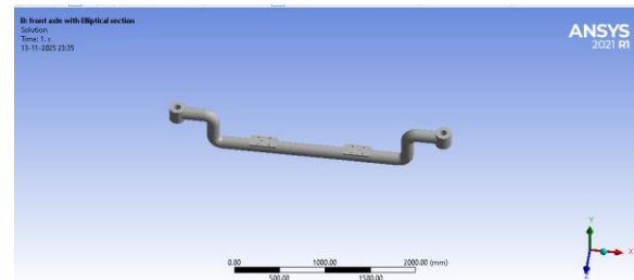
Fig. 9. CAD geometry elliptical section front axle.
