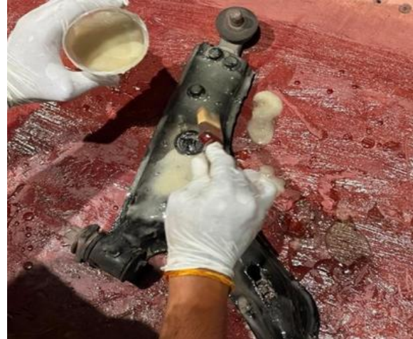
Fig. Glass Fiber layup on the Lower control arm using Resin solution.
