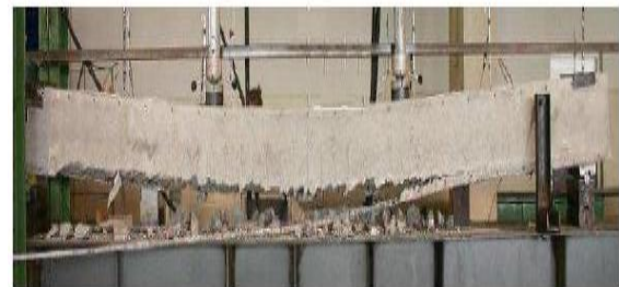
Fig. 3: Cover separation due to intermediate crack debonding
