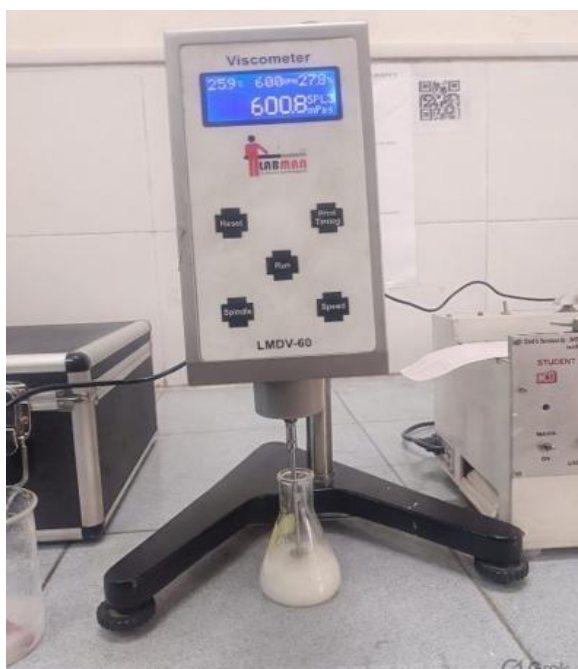
Fig 05: Viscosity determination of formulated herbal face serum using a viscometer
