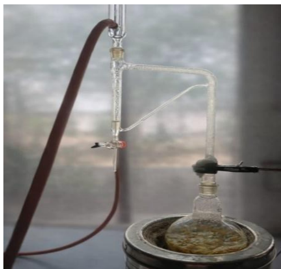
Fig 02: Clevenger apparatus setup for the hydrodistillation of essential oil from orange peel.
