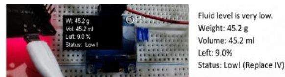
Figure 5: Output of IV Fluid Monitoring System 3
