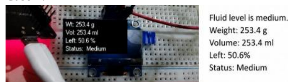
Figure 4: Output of IV Fluid Monitoring System 2
