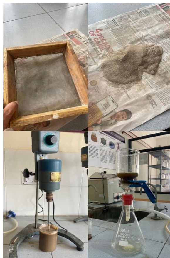
Fig 1: Systematic Extraction of Solanine from Solanum tuberosum Tuber via Acidified Solvent Maceration.[28]
