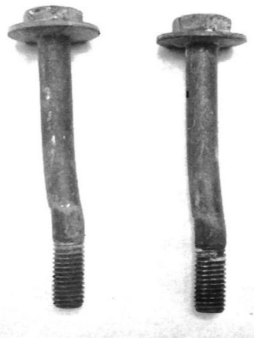
d) bolts after failure
