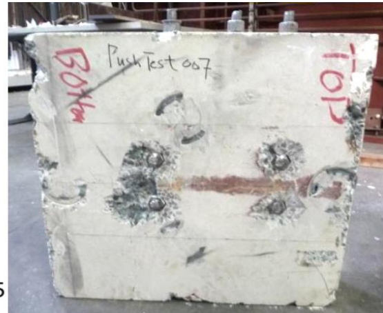
b) concrete slab and bolts after failure
