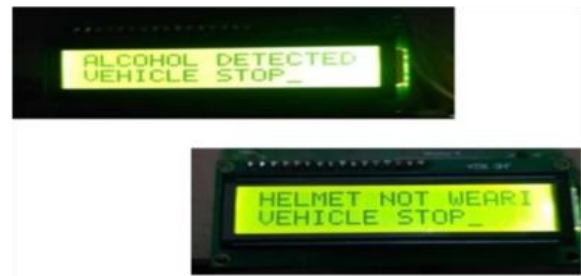
Fig 5 LCD Output of Alcohol Detection System
