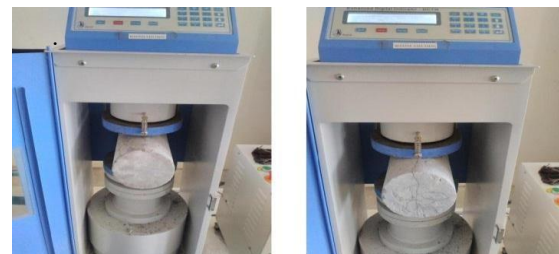
Split tensile testing on cylinder
