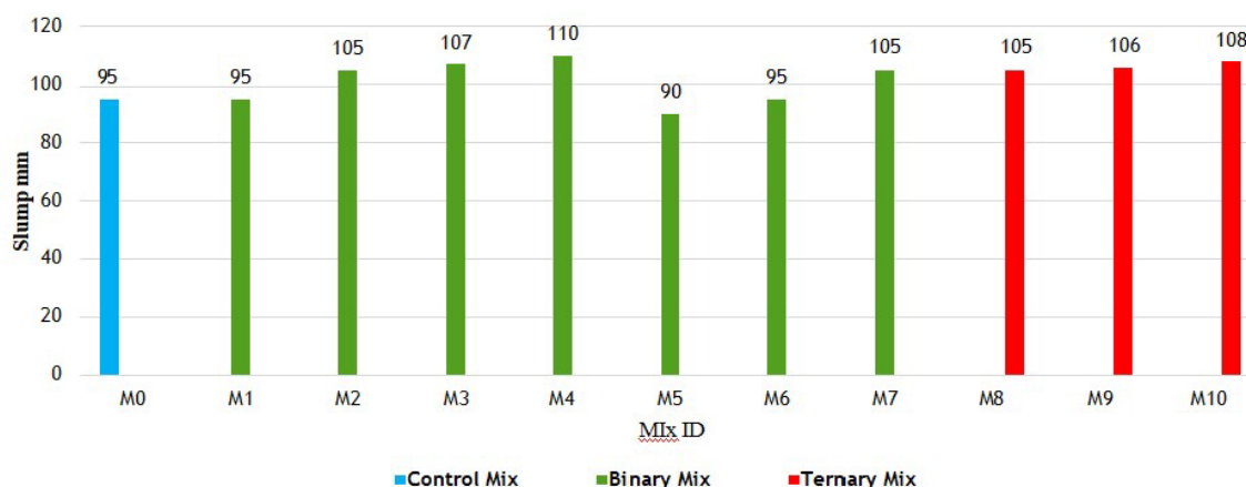
Figure 2. Variation of slump values for control, binary, and ternary concrete mixes incorporating cow dung ash (CDA) and eggshell powder (ESP).
