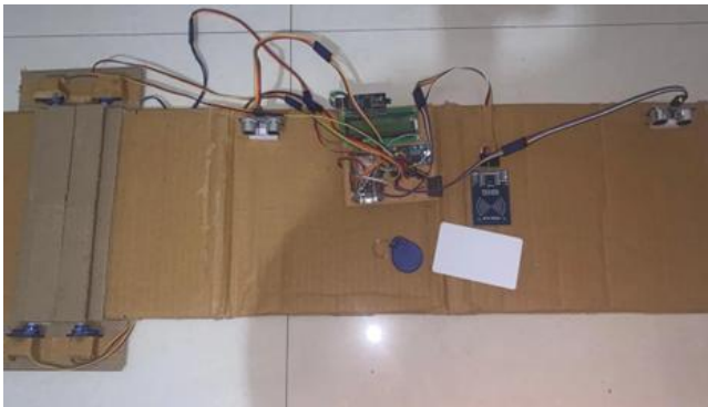
Figure 5. The completed prototype. The two ultrasonic sensors are visible at the two ends of the cardboard road section. The stripboard with the ESP32, the LCD and the buck converter is mounted in the center, and the RFID reader is placed alongside.
