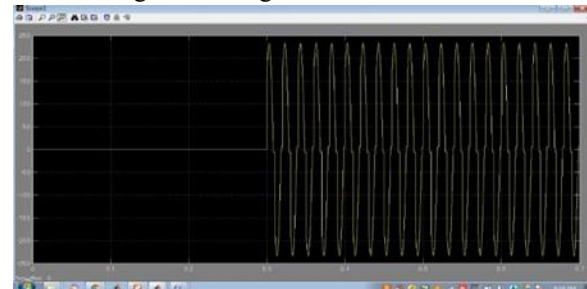
Fig.18. load2 voltage with UPFC under sag mitigation condition
