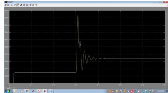
Fig.22. Active power with UPFC in sag condition
