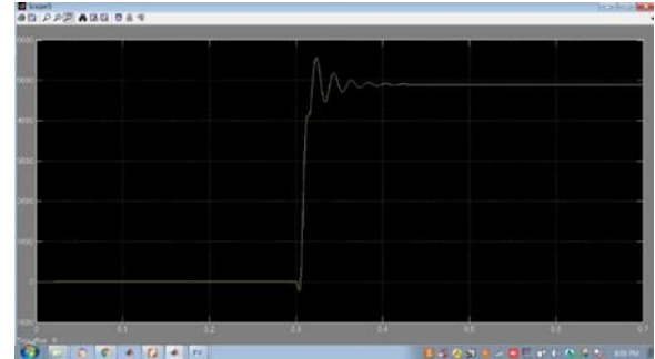
Fig.23. Reactive power with UPFC in sag condition Real and Reactive powers under Swell condition with UPFC
