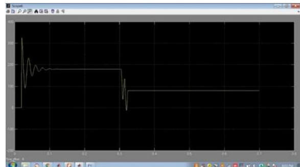
Fig.13 Active power without UPFC under swell condition
