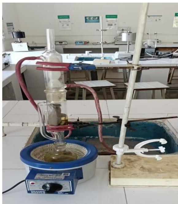
Fig 5 - Soxhlet Extraction of Nerium oleander Powder
