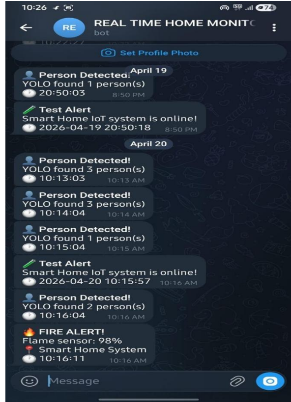
Fig. 8. Telegram bot notification log demonstrating person detection alerts, system online test messages, and critical FIRE ALERT (Flame sensor: 98%).
