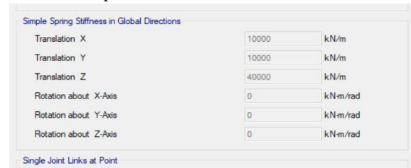
Fig. 11: Point Spring Stiffness Assignment in ETABS (Translational Springs in Global Directions)
