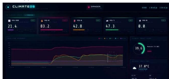
Fig. 4: ClimateOS web dashboard: MQ-135=21.4% (SAFE), MQ-2=83.2% (DANGER), MQ-6=42.8% (SAFE), MQ-7=47.3% (SAFE), MQ-9=0.0%
