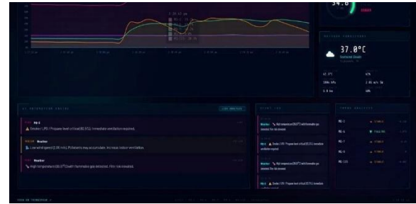
Fig. 5: ClimateOS alert log and trend analysis -- HIGH alert MQ-2 Smoke/LPG critical (82.5%), weather fire-risk advisory (36.9C + flammable gas), low wind speed advisory (2.06 m/s); MQ-6 trend FALLING.
