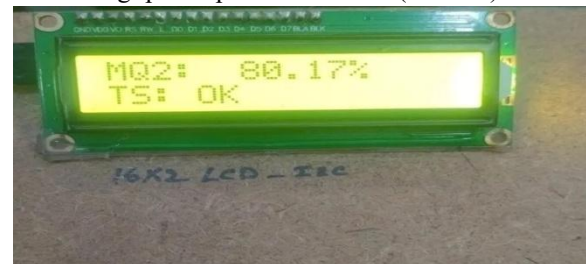
Fig. 2: 16x2 I2C LCD showing MQ-2 reading of 80.17% and ThingSpeak upload status confirmation (TS: OK).
