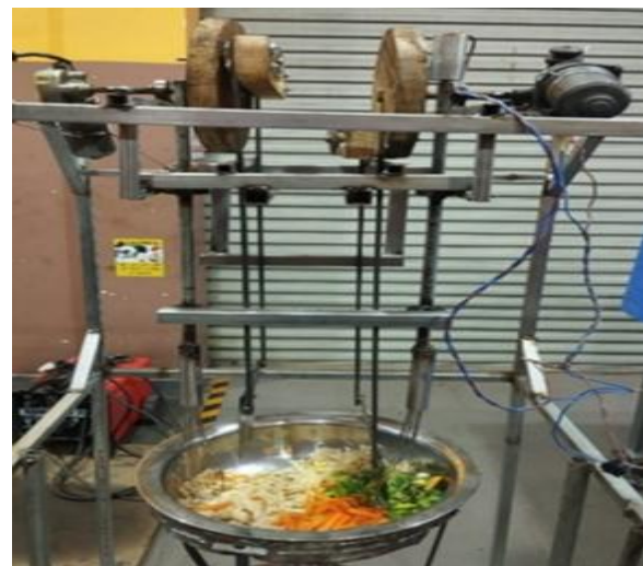
Fig. 5: Prototype of the Semi-Automated Kottu Making Machine
